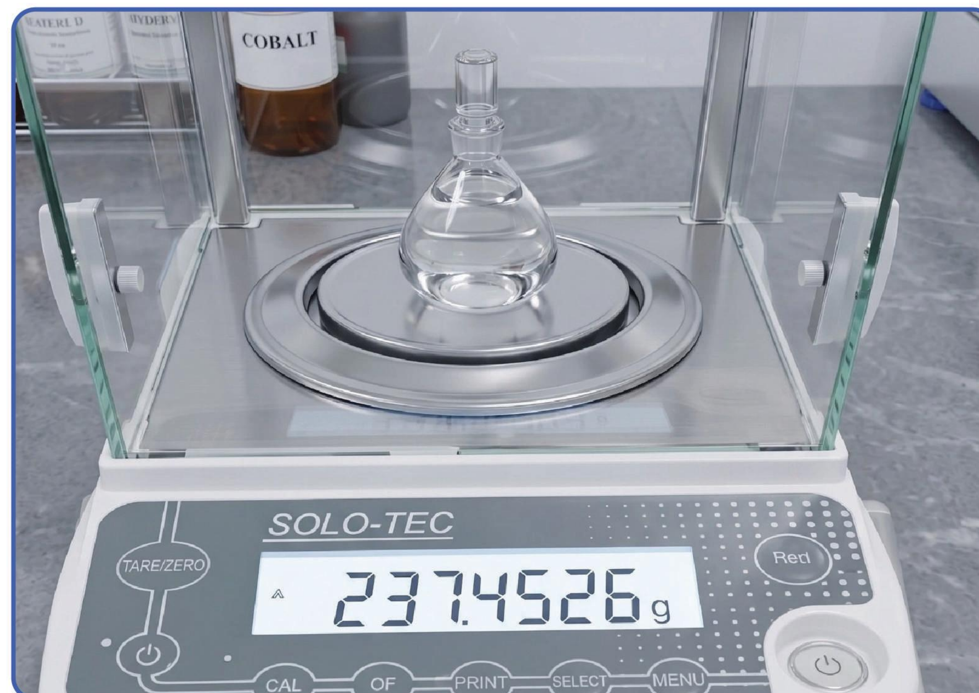
Advanced Resin Density Verification as per IS 6746
