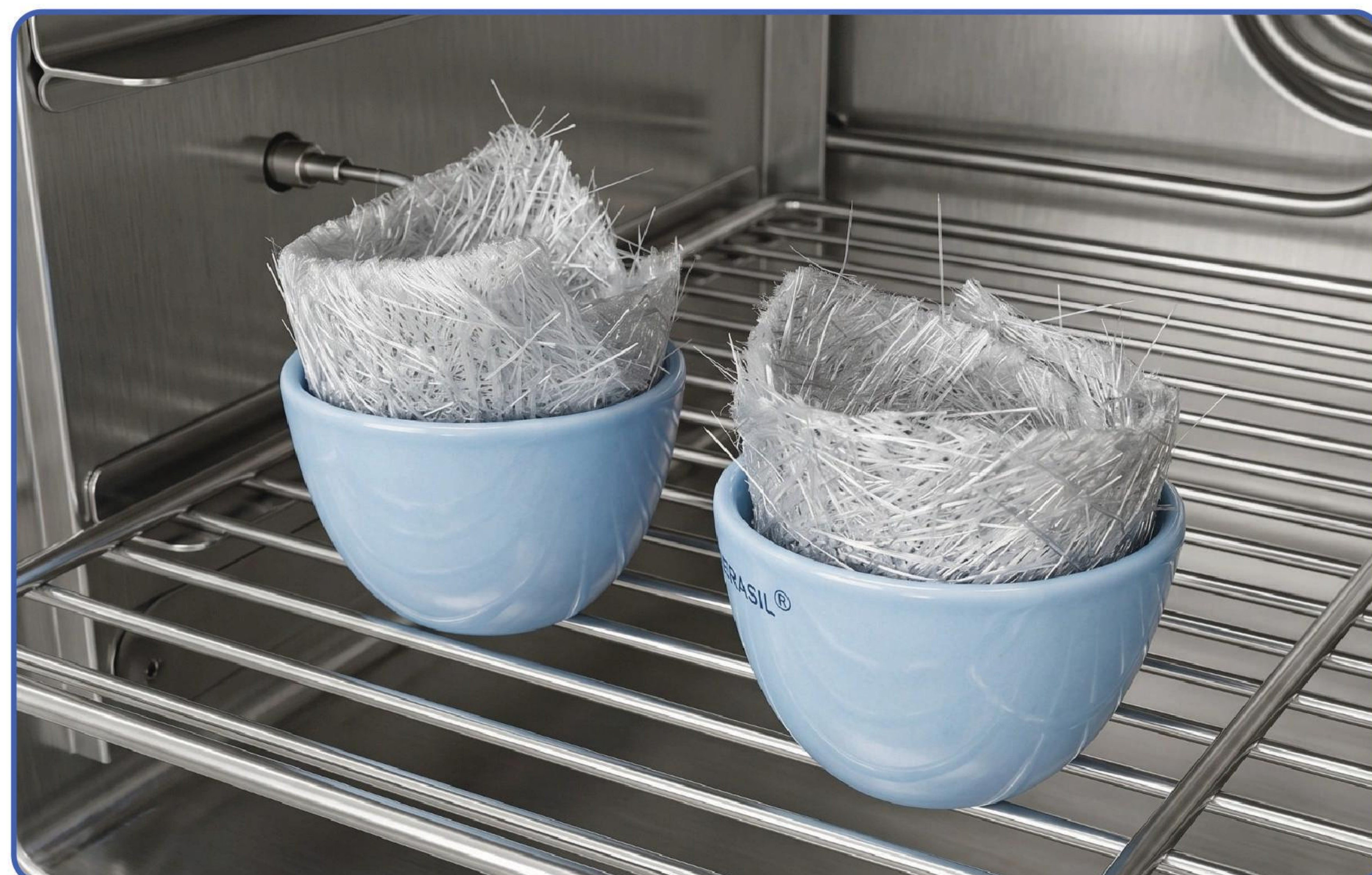
Advanced Loss on Ignition (LOI) Testing as per ASTM D2584
